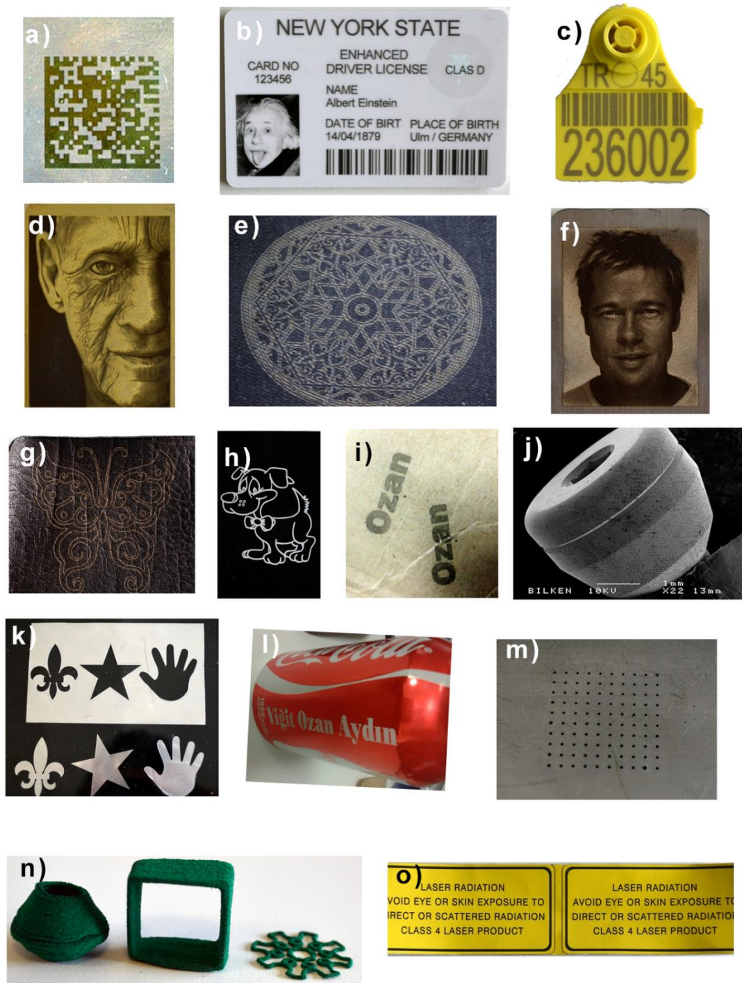
Figure 5.22 Application samples done by developed fiber laser amplifier : marking of a stainless steel a), plastics b) and c), brass d), denim e), stainless steel f), leather g), cart i); day&night marking of aluminium h); precise cutting of a stainless steel k); micromachining of titanium j) ; dye removal of aluminum l); microdrilling of silver m); sintering n); label marking o).
