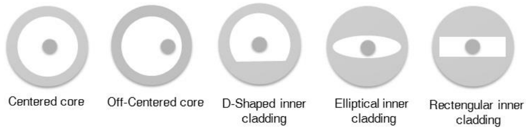
Figure 2.6. Cross sections of different type of double clad fibers.
