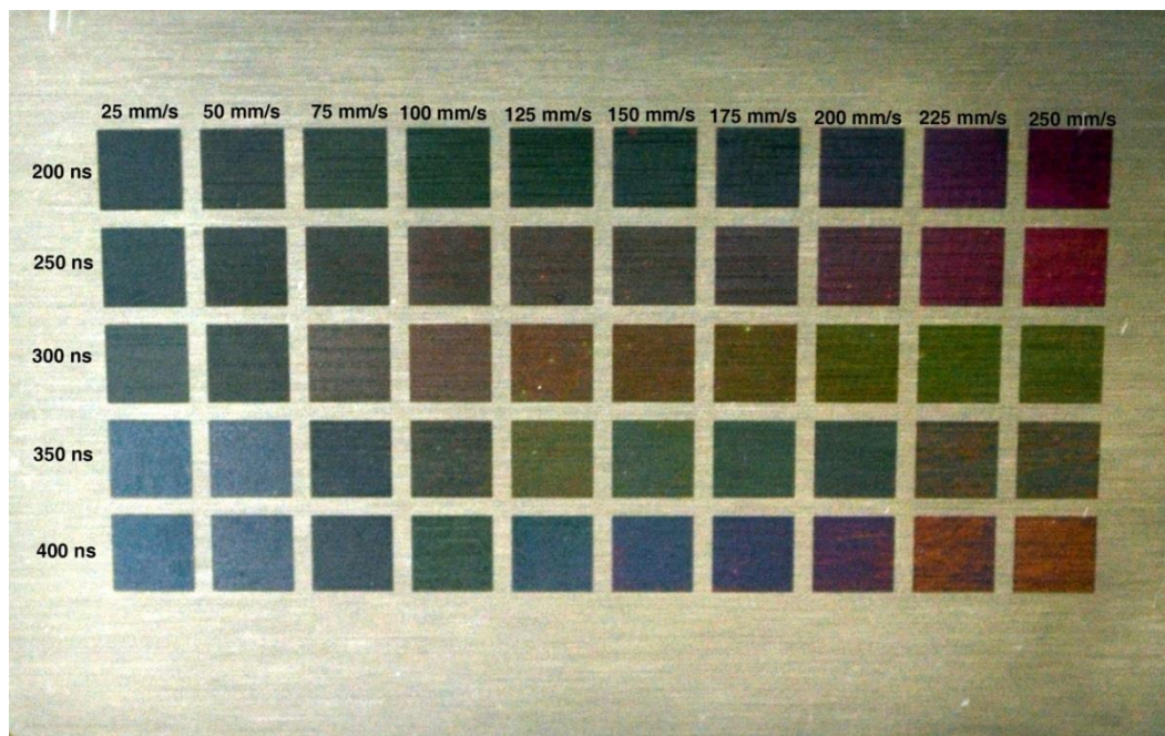
Figure 5.16 Marking stainless steel with varied peak power and constant pulse energy.
