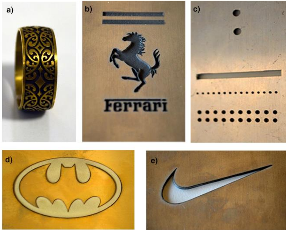
Figure 5.21 Some of the engraving and cutting samples prepared by laser amplifier; engraving of a) 14 carat gold, b) stainless steel, d) brass, cutting of c-d) aluminum.
